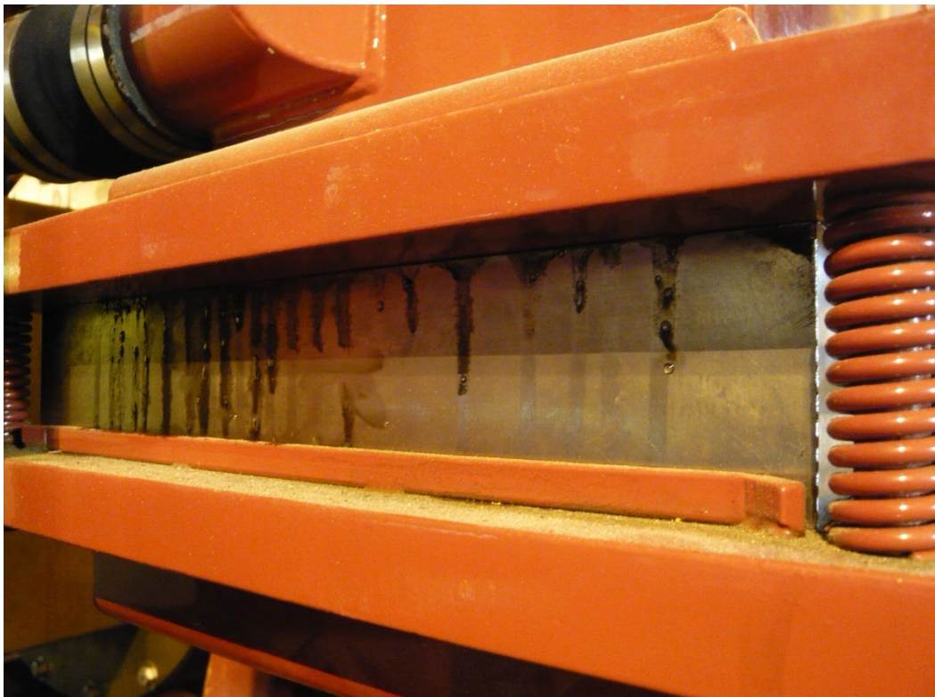
Figure 10 – Condensation Seeping Past the Flame Arresters on Start Up
