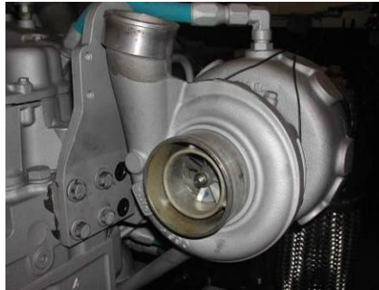
Figure 9 – Turbocharger with Water Cooled Exhaust Housing
