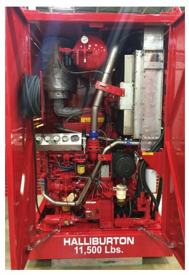
C4.4 wireline unit with remote radiator for slimline fit
