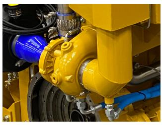
Water-cooled turbocharger and exhaust manifold
