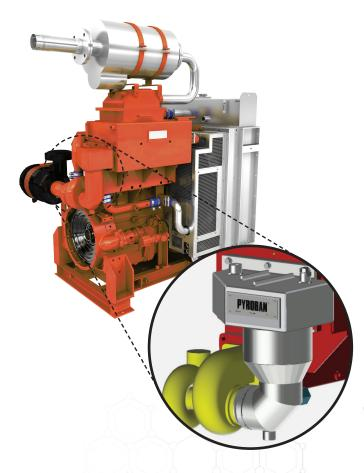
Bolted into the exhaust system between the turbo and gas cooler, ECE flame arrestors are suitable for new, or existing, Pyroban protected turbo diesel engines (100bhp+).
