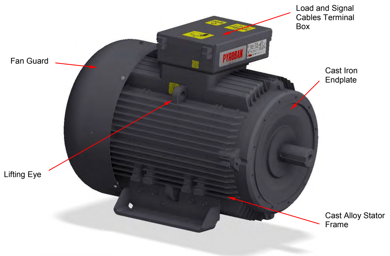
Figure 1 – Alternator General Features
