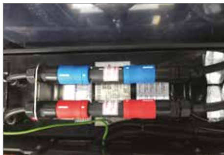
Typical Ex e Battery (Note the specification and certification label on the lid)
