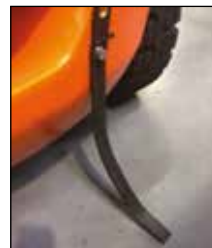
Strap attached to the chassis
