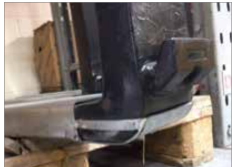
The heel of the fork is left open to allow for periodic inspections
