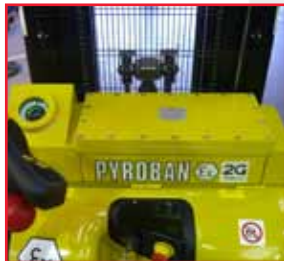
Ex'd' integrated enclosures for arcing and sparking components.
