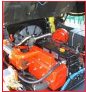
Engine showing Pyroban's exhaust cooling system & components
